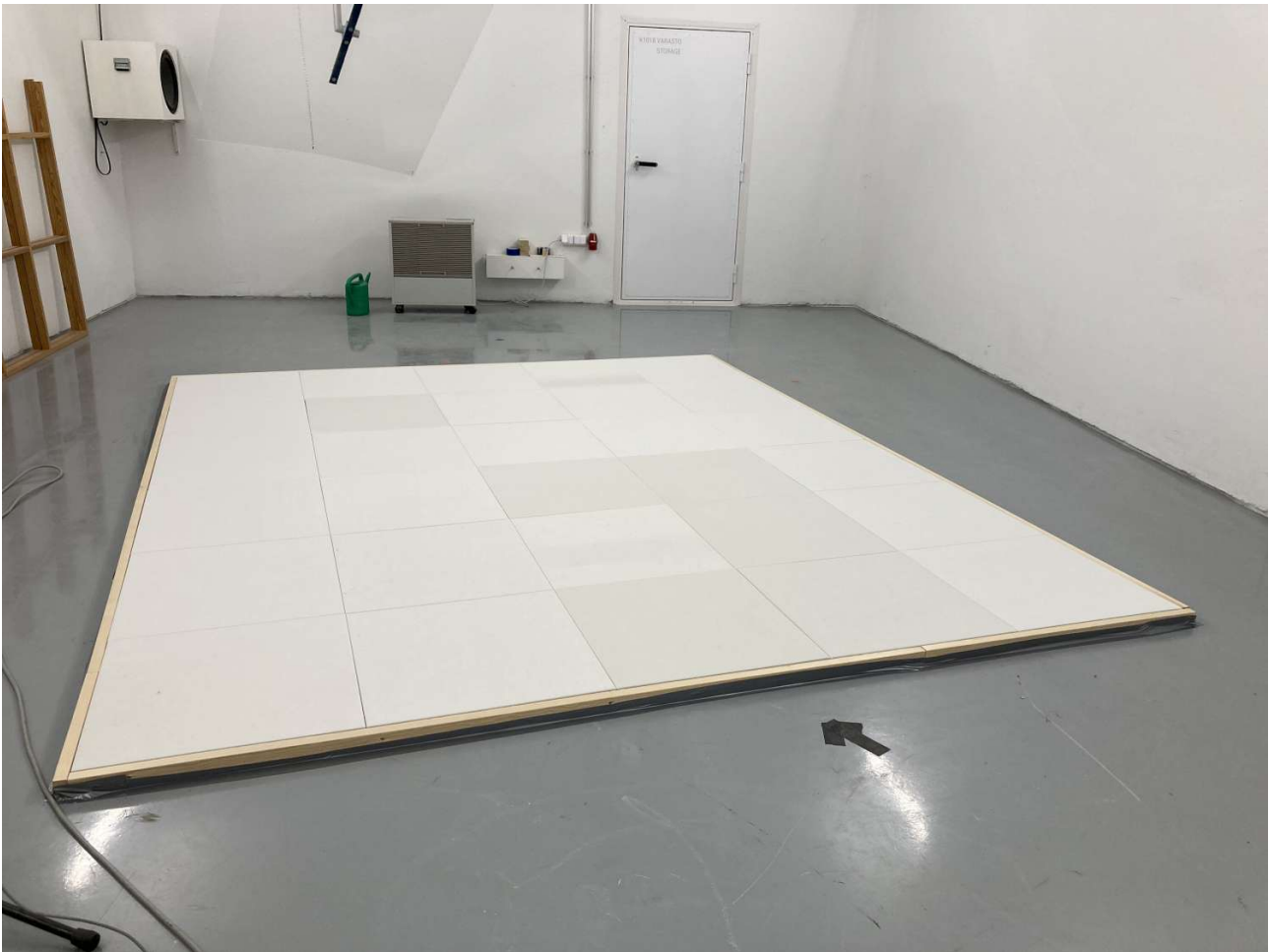
Figure A3.1. The specimen mounted on the floor of the reverberation room.
